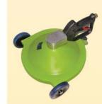
**CaviDome®** has two rotating nozzles to produce a swirling cavitation flame that cleans fouling ahead of the wheels of the dome and under the unit. Negative pressure under the dome holds the device to the surface being cleaned for easy and effective diver control and operation, cleaning a 16" (40 cm) swath in a single pass.
